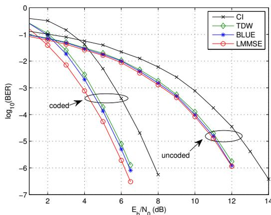
Figure 3: BER performance of the data estimators in the AWGN channel.
