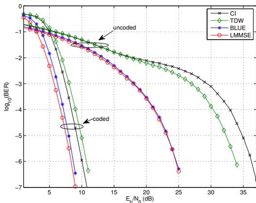
Figure 6: BER performance of the data estimators for channel B.
